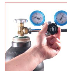
B. Adjust the required charging pressure through the regulation valve. Usually the gauge on the right display the set charging pressure.
