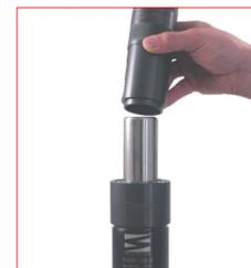
20. Insert the positioning tube ( ) over the rod in contact with the upper side of the assembled bushing, then by the manual press, press down into the cylinder body, the piston rod and the assembled bushing.
