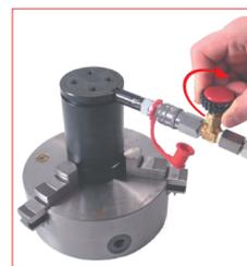
27. When directly charging through the adapter (39DFV01) and desired pressure is reached shut off the hose and bottle valves and disconnect the the quick fit coupling. For an easy and safety work carefully follow the instructions supplied with the charging unit.
