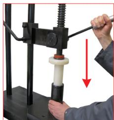
5. Position the anti scratch nylon removal tube on the cartridge (49TN...) then by the manual press (39PM02A) press all down into the body. The retaining ring is now free for an easy removal.
