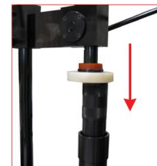
21. By using the manual press (39PM02A) act on the positioning tube to push down the retaining C-ring into its groove. When the C-ring enter into the groove you will hear a "click".
