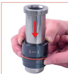
9. Slide off the cartridge from the rod. Discard the cartridge.
