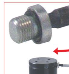
31. Thread the protective screw cap into the charging hole 1/8"G by using the hex key .
