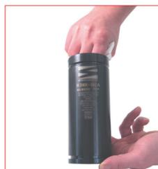
10. Carefully check and clean the cylinder body. If the body show any wear or damage do not use it again and replace it with a new one.
