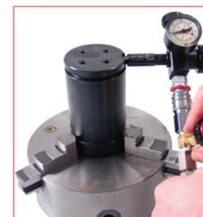
25. Select and assemble the desired charging adapter on the charging unit device (39DMA), thread it on the charging hole and proceed to fill the gas on the desired pressure (Max. 150 if not different specified). Do not exceed the maximum indicated charging pressure.
