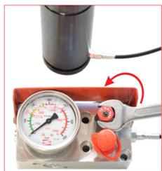
A. To exhaust pressure of hoses cylinders open the discharging valve on the control panel.
