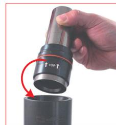
18. Set the positioning tube (49TB...) on the upper part of the cylinder body, then manually insert the piston-rod and the assembled bushing into the positioning tube.
