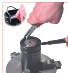
7. By using the C-ring removal tool (58EAR) remove the retaining C-ring by using the appropriate removal tool and pincer (58KNIPEX). Preserve the retaining C-ring for further reassembly.
