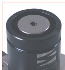
6. Position and clamp the cylinder into a self - centring chuck or a vise.
