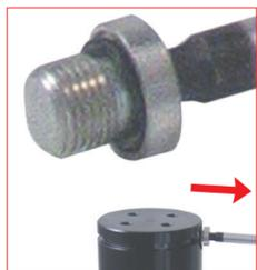
1. Remove the protective screw cap into the charging hole 1/8"G by using the hex key (58CE05). Preserve the protective screw cap for further reassembly.
