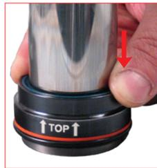
15. Slide down the assembled bushing to the piston shoulder.
