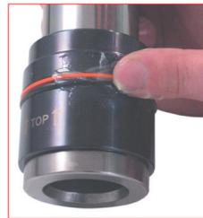
16. Grease the O-ring on the assembled bushing with the specific Special Springs grease.
