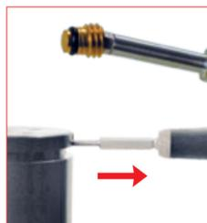
4. Hang and release the one way valve from the hole by using the one way valve removing-setting dynamometric wrench (58CD01). It would be normal some oil leak from the hole when upside down the cylinder.
