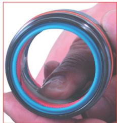
13. Lubricate all the installed components into the assembled bushing with the Special Springs grease.
