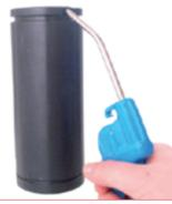
18. Carefully clean the lodging hole of the valve with compressed air and then position the new one way valve supplied along with the maintenance kit. Pay attention to its right position.
