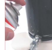
c. Connect the female quick fit on the **D.** It is always recommended to check male quick fit on the panel and open leaks on all connection to and from the gas tap. For an easy and safety the cylinder by using the special gas work carefully follow the instructions
