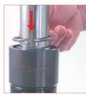
27. Position the retaining C-ring into the conical centring guide tube.
