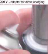
38. It is always recommended to check leaks on the upper side of the cylinders after the maintenance work and before re-using the cylinders by using the special gas detector. 39RFG Special Springs gas detector.
