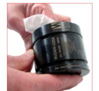
16. Carefully check and clean the cylinder body. If the body show any wear or damage do not use it again and replace it with a new one.
