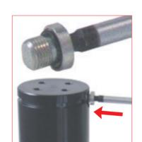
39. Thread the protective screw into the charging hole by using the appro-58CE05 for 1/8G charging port.
