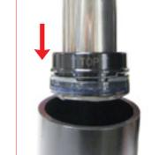
25. Set the positioning tube on the upper part of the cylinder body, then manually insert the piston-rod and the assembled bushing into the position-
