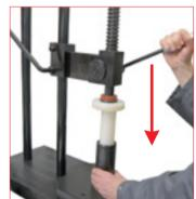
11. Position the anti scratch nylon 11.1. Cross section view of cylinder to 12. Position and clamp the cylinder removal tube (49TN...) on the bush then by the manual press (39PM02A) press all down into the body. The retaining ring is now free for an easy
