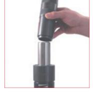
26. Insert the positioning tube over the rod in contact with the upper side of the assembled bushing, then by the manual press, press down into the cylinder body, the piston rod and the assembled bushing.
