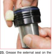
assembled bush with the specific Special Springs grease.
