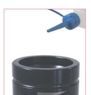
24. Lubricate inside the cylinder body with the specific Special Springs oil supplied with the repair kit. Pay attention to the quantity as indicated for each cylinder model.
