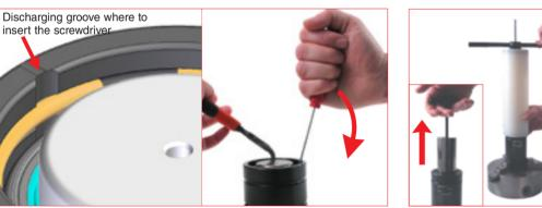
13. By inserting the screwdriver on the appropriate discharging groove, between the retaining ring and the body border, remove the ring as indicated. Use the pliers (58KNIPEX) to avoid that the ring comes out sharply. Use the flat screwdriver 2.5 x 75.
