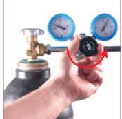
31. Adjust the required maximum pressure trought the regulation valve. The gauge on the right will indicate the maximum allowed pressure to charge the cylinder. 39R... pressure reducer.
