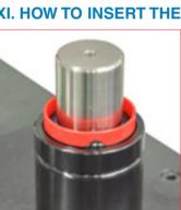
40. Direct the V-shaped discharging section, as shown in the image. Place the Over Stroke Marker by aligning the indicator tooth with the discharging grooves.
