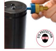
8. Thread DDS discharging device on the charging port then exhaust completely the pressure. Point away from the operator for maximum safety. 39DDS01A BLUE side for M6 hole GOLD side for 1/8"G hole
