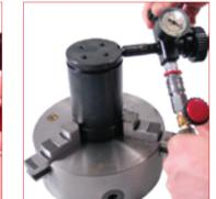
33. Once reached and stabilized the desired pressure, for an easy and safe operation carefully follow the instructions supplied with the charg-
