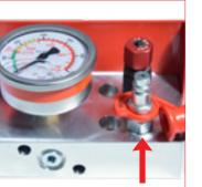
A. After positioning and hosing all the cylinders, proceed through the quick fit device trough the control panel for charging all the cylinders. Make sure that the discharging valve is closed properly (15 Nm).
