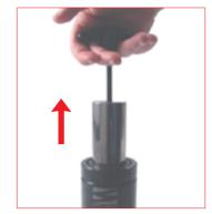
29. Manually extract the assembly piston-rod/bush untill it rests against the C-ring
