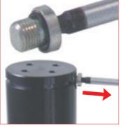
7. Remove the charging plug from the charging hole by using the appropriate tool. Preserve the charging plug for further
