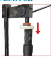
28 Insert the positioning tube in contact with the retaining C-ring, then by the manual press, press down the retain-
