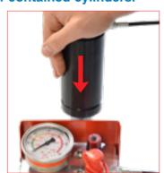
B. Be sure the pressure is completley exhausted by pressing down the piston rod into the cilynders body.
