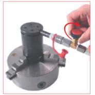
**34.** When directly charging throught **35.** Thread and relase the the adapter, after the desired pressure is reached, shut off the hose and bottle valves and disconnect the quick fit coupling.
