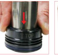
22. Slide down the assembled bush to the piston shoulder
