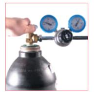
30. Check the correct assembly of the pressure regulation valve on the gas bottle, then open the main tap. The gauge on the left will indicate the
