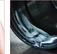
25. Lubricate the bottom grooves 26. Lubricate the top of the rod using using the Special Springs grease. 590GRASSO Special Springs grease
