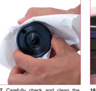
17. Carefully check and clean the bottom base, blowing inside pressurized air to remove residuals from the dual-ring groove and charging port. If the bottom base shows any wear or damage DO NOT use it again and replace it with a new one.
