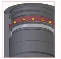
**13.** While removing the sealing and guiding elements, pay attention NOT to damage the internal lodging grooves.
