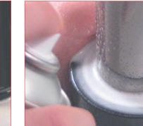
E. It is always recommended to check leaks on the upper side of the cylinders after the maintenance work and before re-using the cylinders by using the special gas detector. 39RFG Special Springs gas detector.
