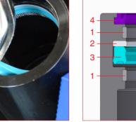
22. Install in the same groove the 23. Cross-section view of a correct gas seal. If necessary, use the pliers assembling. avoiding damaging the lips of the gas
