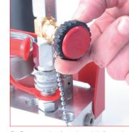
C. Connect the female quick fit on the male quick fit on the panel and open the gas tap. For an easy and safe operation carefully follow the instructions supplied with the charging unit. 39DMCPVA control panel charging unit.
