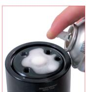
**39.** A more precise force control can 40. It is always recommended to be carried out by using the digital check leaks on the charging port after the maintenance work and before re-using the cylinders by using the special gas detector. 39RFG Special Springs gas detector.
