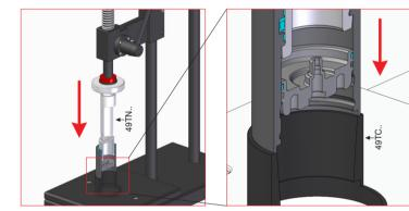
10. Press the rod inside the body using the manual press (39PM02A), the the rod out of the cylinder body. suitable anti-scratches nylon tube (49TN..) and the positioning tube (49TB..).
