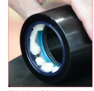
**23.** Lubricate all the internal elements using the Special Springs grease 590GRASSO Special Springs grease
