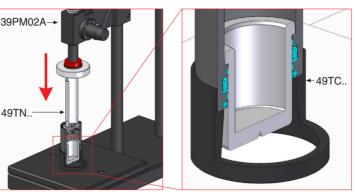
5. Press the bottom base inside the body using the manual press (39PM02A), the suitable anti-scratches nylon tube (49TN .. ) and the positioning tube (49TC) for an easy removal of the retaining C-ring.
