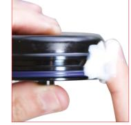
**24.** Lubrificate all the installed elements using the Special Spring grease. 590GRASSO Special Springs grease
