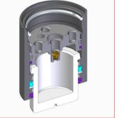
30.1. Cross section of correct retaining-ring assembling. ALWAYS check the correct and complete positioning of the c-ring into the proper groove.
