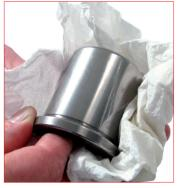
16. Carefully check and clean the rod. If the rod shows any damage, wear or scratch DO NOT use it again and replace it with a new one
