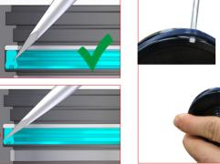
13.1 Remove the gas seal without scratching the internal lodging grooves with the screwdriver. groove.
