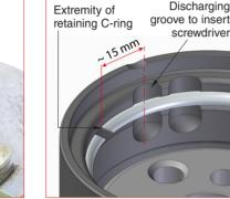
8. Position the extremity of the retaining ring at about 15 mm from the groove centre.
