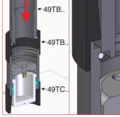
Using the manual press 30. (39PM02), the proper anti-scratches nylon tubes (49TN .. ) and the positioning tube (49TB .. ), press into the original position the retaining C-ring. The correct positioning will make a "click" sound.
