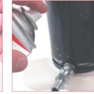
**D.** It is always recommended to check leaks on all connections to and from the cylinder by using the special gas detector 39RFG Special Springs gas detector.
