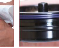
18. Assembly the dual ring on the bottom base as shown on the picture.Pav attention NOT to twist the dual-ring.
