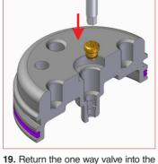
original position. Screw it by using the torque wrench for one way valve untill a "ĊLICK". 58CD01 torque wrench for one way valve
