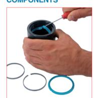
11. Example with the bottom base and 12. Remove from the cylinder body all the seals and guiding elements.
