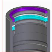
20. Assembly all the gas seals and guides (as shown on the picture) on the following order: 1 Guiding ring 2 Back-up rod seal 3 Rod seal 4 Rod wiper
