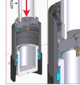
29. Using the manual press (39PM02), the proper anti-scratches nylon tubes (49TN .. ) and the positioning tube (49TB..), press into the original position the bottom base, leaving enough space for the assembly of the retaining C-ring.
