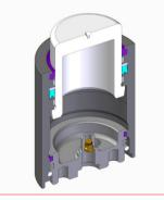
**31.** Use a pressurized air to bring into a correct position the bottom base and the rod.
