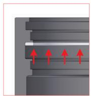
21. Once the back up ring is installed inside the groove, push it upword. seal ring. 58KNIPEX pliers
