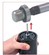
1. Remove the protective plug from the charging hole by using the appropriate tool. Preserve the protective plug for further reassembly. 58CE05 for the 1/8 G port. 58CE03 for the M6 port.
