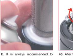
check leaks on the upper side of the cylinders by using the special gas 39RFG Special Springs gas detector.
