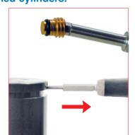
4. Hang and release the one way valve from the hole by using the appropriate tool. It would be normal some oil leak from the hole when upside down the cylinder. 58CD01 one way valve removingsetting dynamometric wrench.
