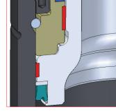
29. Cut off with all components correctly assembled.
