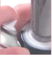
42.1. It is always recommended to check leaks on the upper side of the cylinders after the maintenance work and before re-using the cylinders by using the special gas detector. 39RFG Special Springs gas detector.
