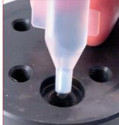
31. Upside-down the cylinder and drop the lubricating oil supplied with the kit. Please do not exceed the volumes as indicated in the tab.
