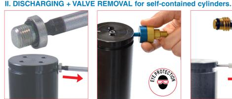
2. Remove the protective screw cap from the charging hole by using the appropriate tool. **58CE05** for the 1/8 G port. 58CE03 M6/3 for the M6 port.
