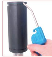
19. Carefully clean the lodging hole of the valve with an airgun and then position the new one way valve supplied along with the maintenance kit. Be care on the right position of it.
