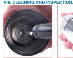
17. Carefully check and clean the cylinder body. If the body show any wear or damage do not use it again and replace it with a new one.
