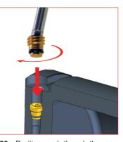
20. Position and thread the one way valve into the hole by using the appropriate special dynamometric tool. Torque force required maximum 0,6 Nm. Do not exceed the maximum torque force indicated to not damage the one way valve. 58CD01 dynamometric wrench.
