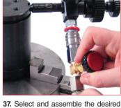
charging adapter and thread it on the charging port. For an easy and safety work carefully follow the instructions supplied with the charging unit. DO NOT exceed the maximum pres-
