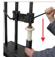
11. Position the anti scratch nylon 12. Cylinder section with piston/rod removal tube on the cartridge then press down into the body for about 25 mm to set free the retaining C. 39PM02A manual press.
