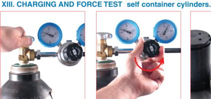
**36.** Adjust the required maximum pressure trought the regulation valve. The gauge on the right will indicate the maximum allowed pressure to charge the cylinder. 39R... pressure regulation valve.
