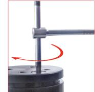
33. Lock up the safety device by using the appropriate tool. 58CE05 hex key.
