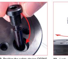
**32.** Position the safety device OSPAS into the proper hole located in the cylinder bottom. It is severely forbidden to press the piston-rod into the body when the safety device OSPAS is positioned. High risk to damage and compromise the functional of the safety device.
