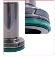
21. Assembly into the proper groove the new guide and the new piston Pay the best attention to not damage the seal as well as to the right positioning.
