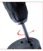
6. To remove the safety device OSAPS it is necessary to remove first the aluminium seal from the hex hole of the screw. Use the special drill hit. included in the maintenance kit, and mount it on a small hand drill.
