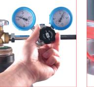
B. Adjust the required pressure on the regulation valve on the bottle. The gauge on the right will indicate the maximum allowed pressure to charge the cylinders.
