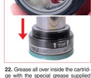
ge with the special grease supplied with the kit and manually press the pre-assembled cartridge into the rod and slide down to the piston shoulder. Pay the best attention to the right orientation of the cartridge.
