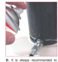
check leaks on all connection to and from the cylinder by using the special 39RFG Special Springs gas detector.
