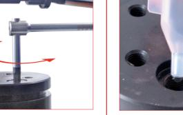
8. Remove the safety device OSAPS by using the appropriate tool and take Preserve the safety device OSAPS
