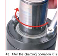
recommended to double check the right docking of the upper ring nut on the body by using the appropriate compass wrench. 58CC... compass wrench.
