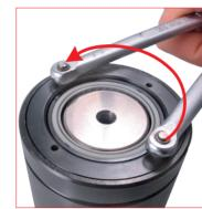
10. Remove the upper ring nut on the body by using the appropriate wrench
