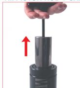
15. Manually extract together piston/ rod/cartridge from the cylinder body. It would be required some strain for certain models.
