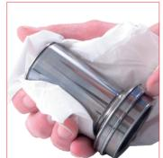
18. Carefully check and clean the piston-rod. If the piston rod shows any damage, wear or scratch do not use it again and replace it with a new one.
