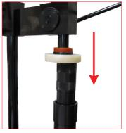
**27.**Insert the positioning tube in contact with the retaining C-ring , then by the manual press, press down the retaining C-ring into the groove When the C-ring enter correctly into the groove you will hear a loud like "CLICK". 49TB... conical centring guide tube. 39PM02A manual press.
