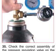
the pressare regulation valve on the gas bottle, then open the main tap. The gauge on the left will indicate the bottle pressure.
