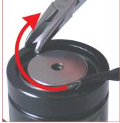
14. Remove the retaining C-ring by using the appropriate removal and pincer. Preserve the retaining C-ring for further reassembly. 58EAR C-ring removal tool. 58KNIPEX pincer.
