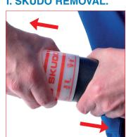
1. Manually remove the protective cap SKUDO. Do not use tools. For certain models the operation will require a certain strain. Preserve the protective cap SKUDO for further reassembly.
