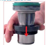
16. Slide off the cartridge from the rod and remove seal and guide from the piston. Discard all of them
