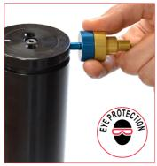
3. Thread DDS discharging device on the charging port then exhaust completely the pressure. Point away from the operator for maximum safety. 39DDS01A BLUE side for M6 hole GOLD side for 1/8"G hole
