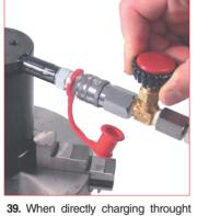
the adapter and desired pressure is reached shut off the hose and bottle valves and disconnect the the quick fit coupling. For an easy and safety work carefully follow the instructions supplied with the charging unit. **39DMCPVA** charging unit.
